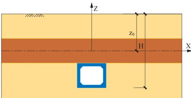
**Fig. 1.** New tunnelling below existing tunnel without clearance in between.
