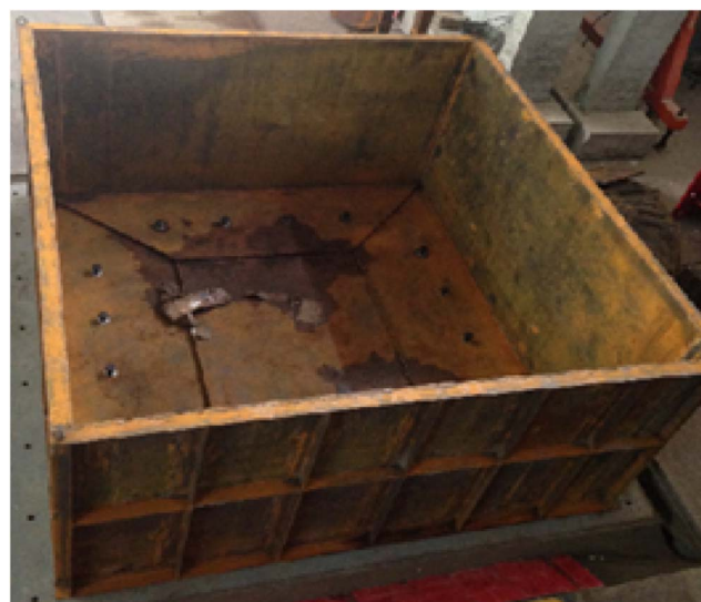
(a) Model container without strengthen slant support
