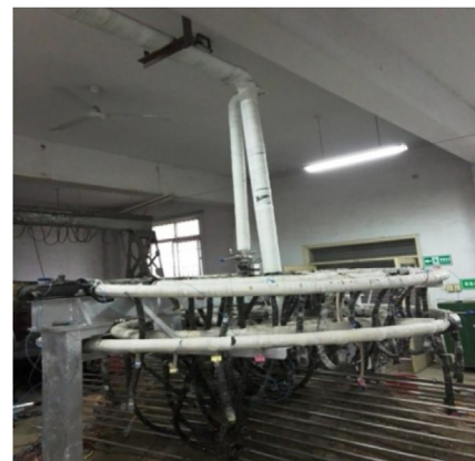
(b) External circulation system
