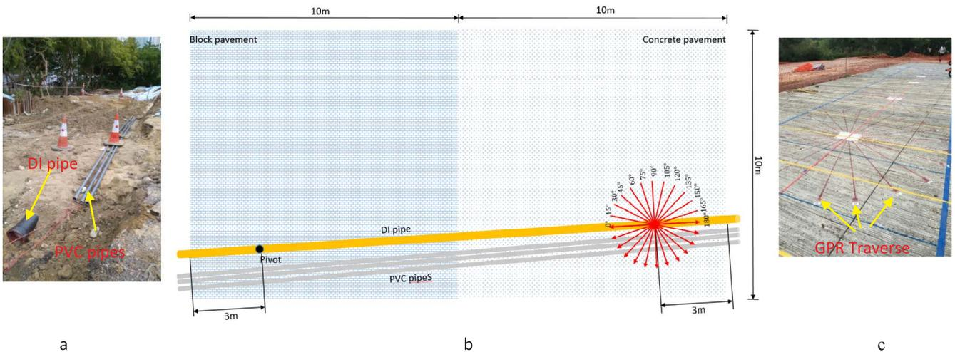
Fig. 2. Survey layout of the test site. Remark: the PVC bundle were put deliberately to observe the effects of small and weak scatterers on the reflection of D.I. pipe.
