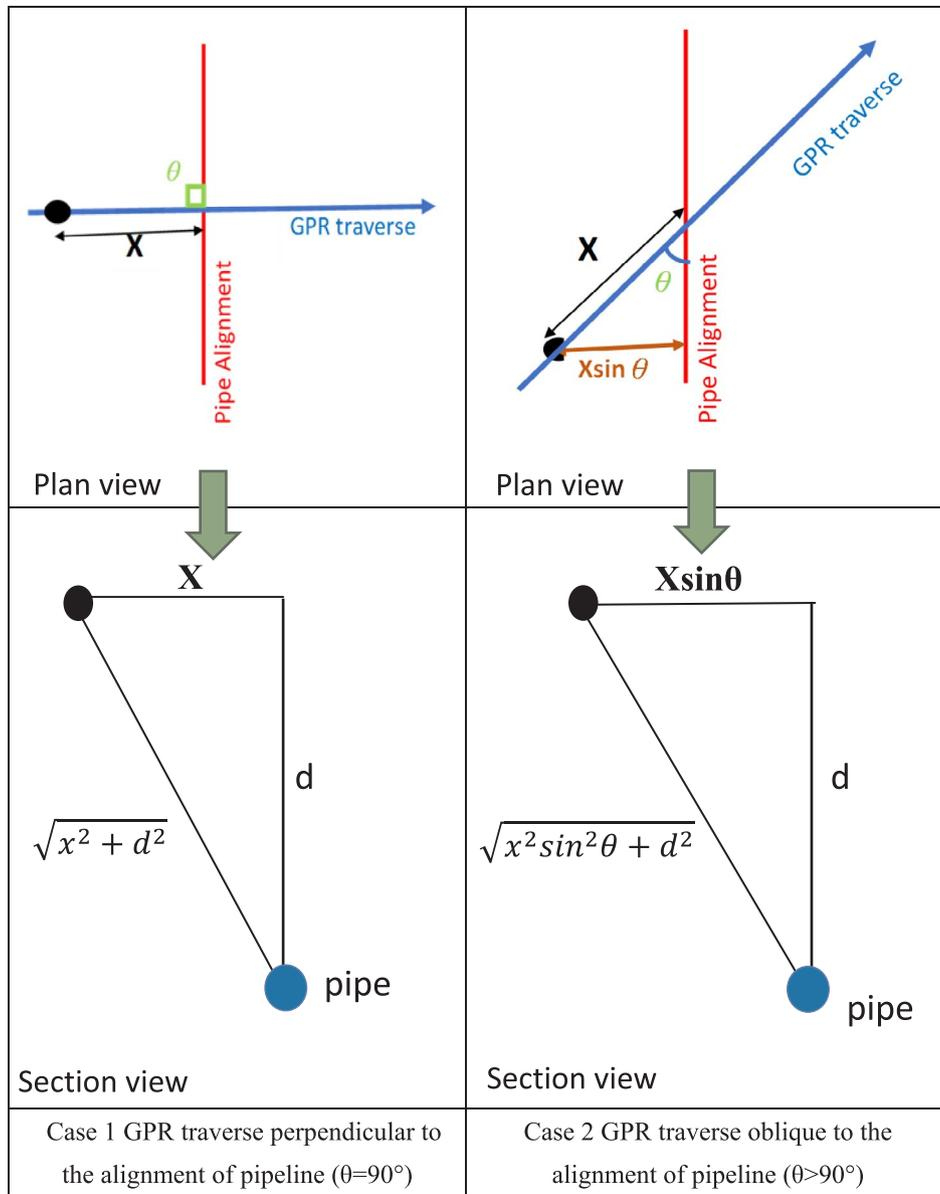
Fig. 1. Illustration of oblique angle on the GPR traverse.
