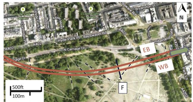
Fig. 2. Alignment of Crossrail tunnels beneath Hyde Park and location of Section F with surface and subsurface instrumentation (aerial photo courtesy of Google maps).
