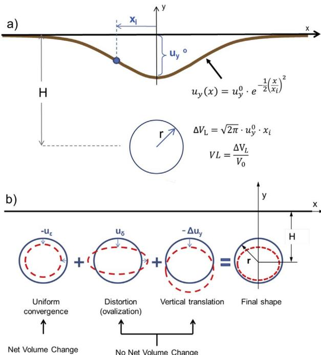
Fig. 1. Interpretation of ground movements; (a) by empirical methods (after Peck, 1969), (b) deformation modes around tunnel cavity (after Whittle and Sagaseta, 2003).
