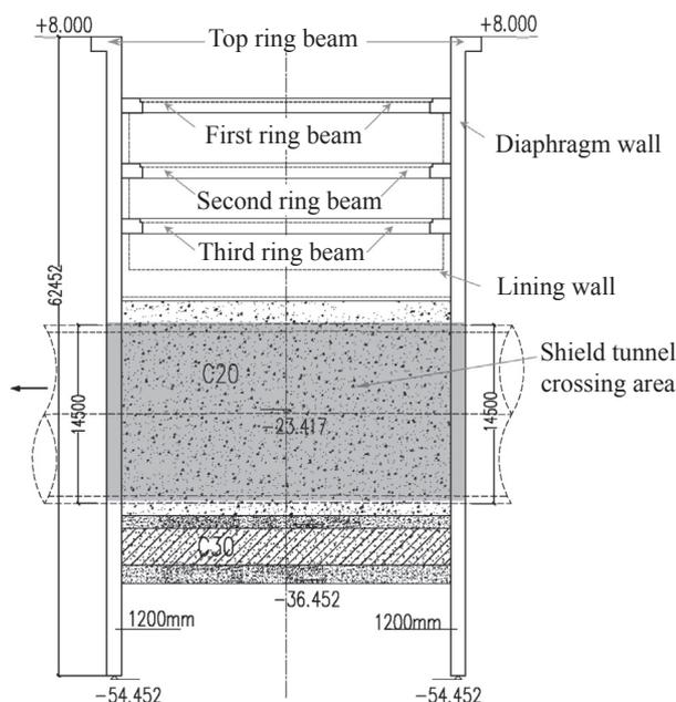
Fig. 1. Profile sketch of the Meizizhou ventilating shaft.
