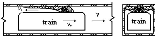
Fig. 1. A train on fire while moving in the forward direction in a subway.
