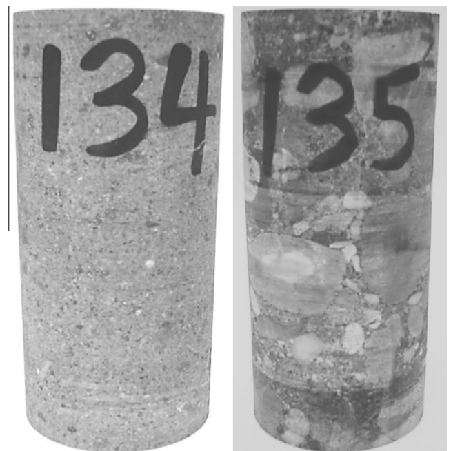
Fig. 1. Examples of two different end-members of conglomerate grain structure in laboratory testing samples.
