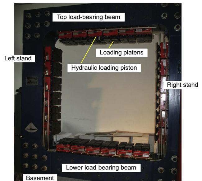
Fig. 1. Photograph of the YDM-C geological disaster simulation testing machine.
