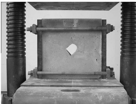
Fig. 2. A cement mortar tunnel model and its loading device.
