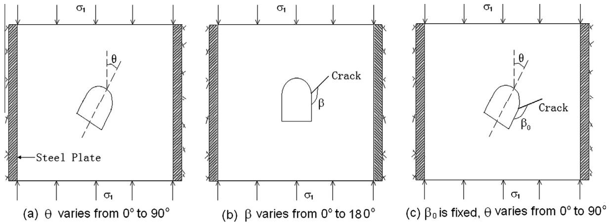
Fig. 1. Three test models of tunnels.
