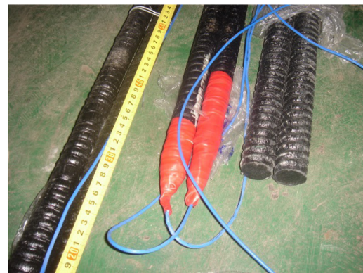
(b) GFRP bar embedded with FBG sensors
