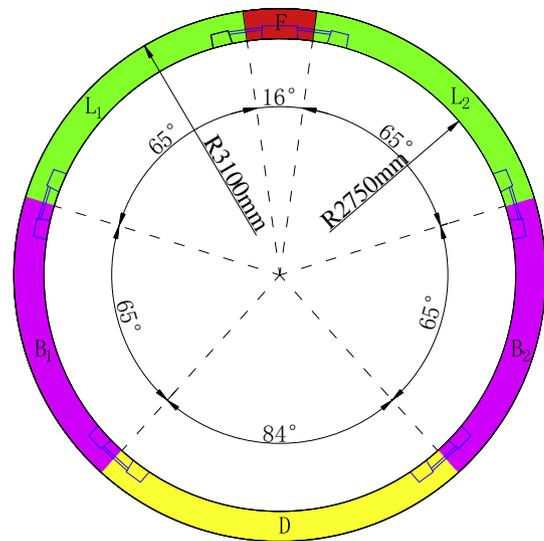
Fig. 1. The structure of tunnel lining.
