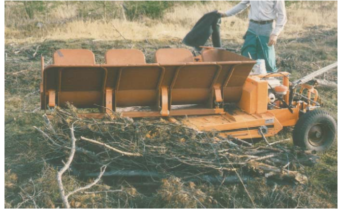
Fig. 1. A simple, manually fed test rig for making bundles.
