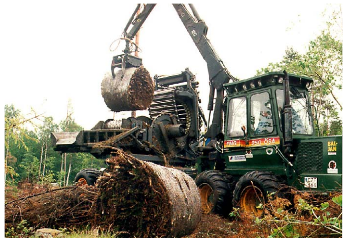
Fig. 3. Machine for baling of logging residues (Bala Press).
