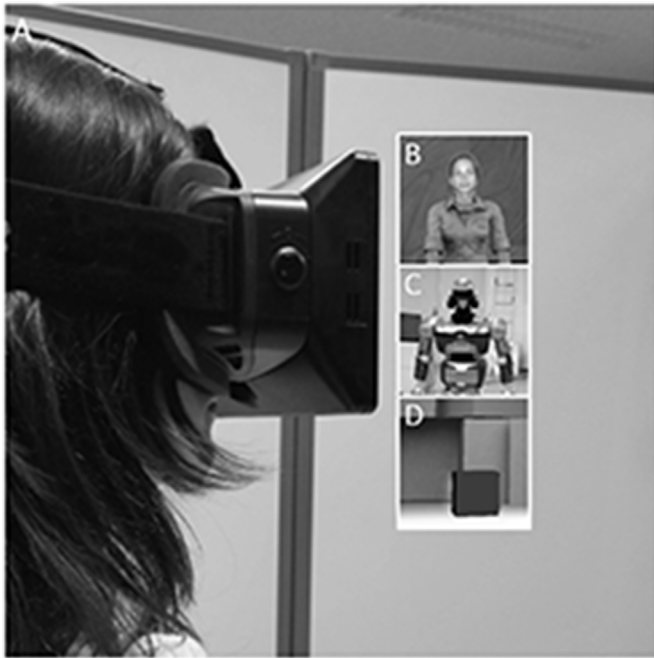
Fig. 1. Mediated embodiment process. Users wear a head-mounted display (A) which provides first-person audiovisual perspective from the avatar body and blocks vision from the physical world. Users embody an avatar in virtual reality (B) or in a physical environment (C) and experience its body and its surroundings in first person. Avatars can also be non-anthropomorphic living beings or objects (D).
