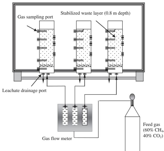
**Fig. 1.** Schematic of waste lysimeter experiment.
