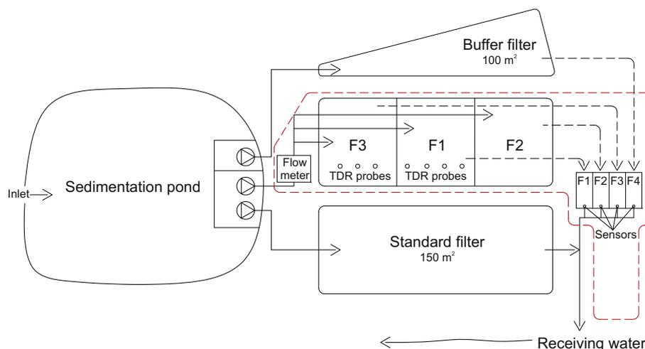
**Fig. 1.** Schematic setup of constructed wetland at Riesweiler with the lava sand filters F1, F2 and F3.
