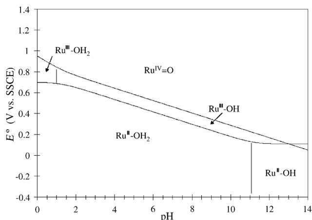
Fig. 1.  $E_{1/2}$  vs. pH or Pourbaix diagram of [Ru(bpea)(bpy)(H<sub>2</sub>O)]<sup>2+</sup>. The pH-potential regions of stability for the various oxidation states and their dominant proton compositions are indicated by using abbreviations such as Ru<sup>II</sup>OH<sub>2</sub>, for example for [Ru<sup>II</sup>(bpea)(bpy)(H<sub>2</sub>O)]<sup>2+</sup>. The  $\text{p}K_{\text{a}}$  values are shown by the vertical solid lines in the various  $E$ -pH regions.
