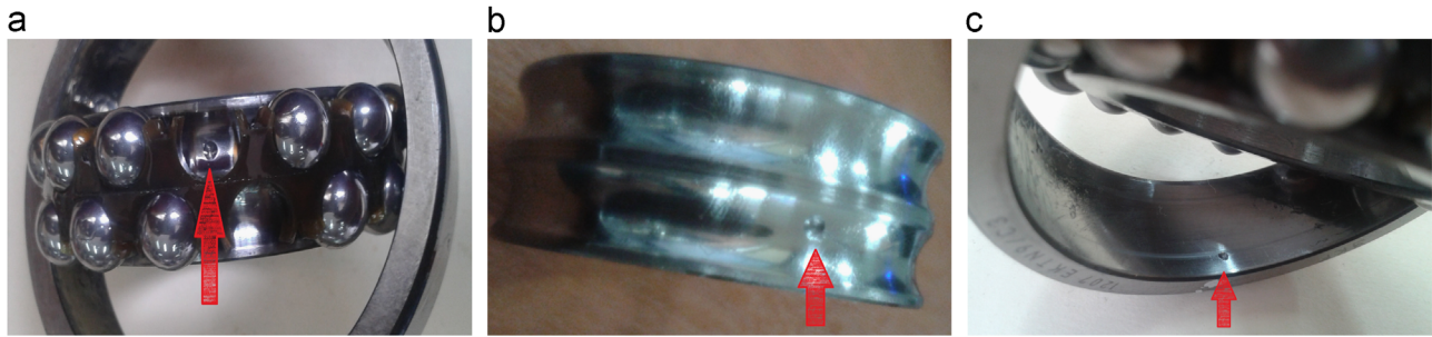
Fig. 1. Examples of the three basic types of bearing faults actually studied in this work: (a) ball bearing fault, (b) inner race fault, and (c) outer race fault.
