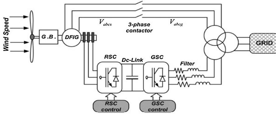
Fig. 1. Schematic diagram of the grid connected DFIG.
