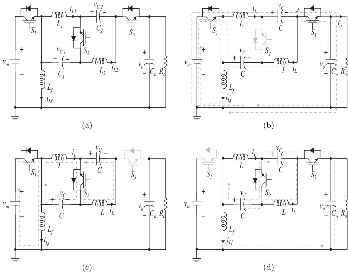
Fig. 1. (a) Buck-boost-based TSTS-ZSI proposed in [8]; (b)–(d) three possible states for the TSTS-ZSI: (b) State 1:  $S_1$  and  $S_3$  are on,  $S_2$  is off; (c) State 2:  $S_1$  and  $S_2$  are on,  $S_3$  is off; (d) State 3:  $S_2$  and  $S_3$  are on,  $S_1$  is off.
