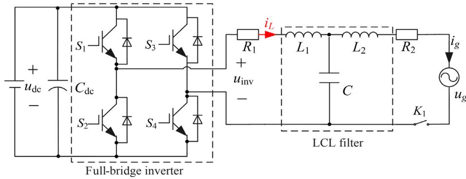
Fig. 1. Structure of single-phase grid-connected inverter with LCL-filter.
