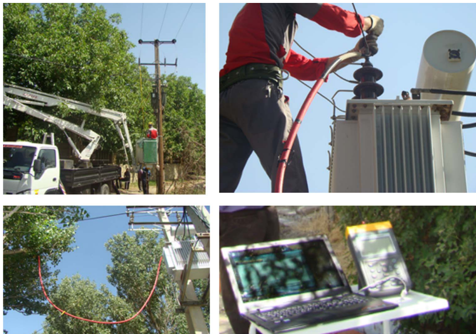
Fig. 2. Test configuration for HIF on live Walnut.
