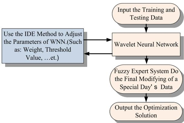
**Fig. 1.** The flowchart of combined improved Differential Evolution–Wavelet Neural Network and Fuzzy Expert System model do the load forecasting of air-conditioning.
