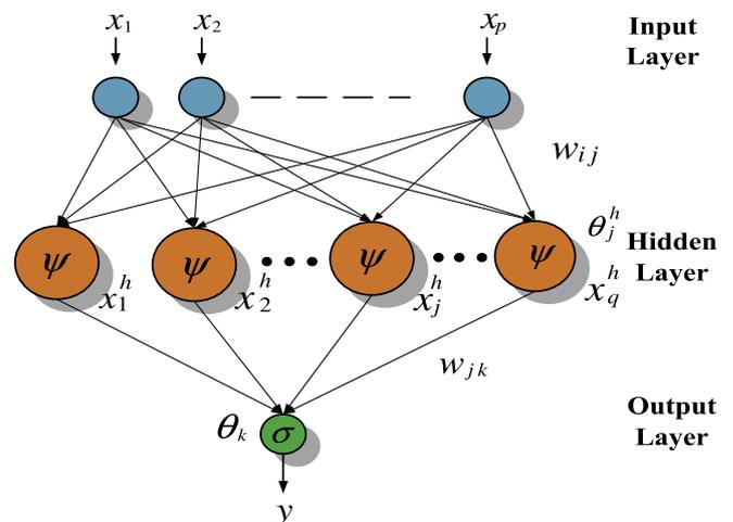
**Fig. 2.** The construction figure of Wavelet Neural Network.
