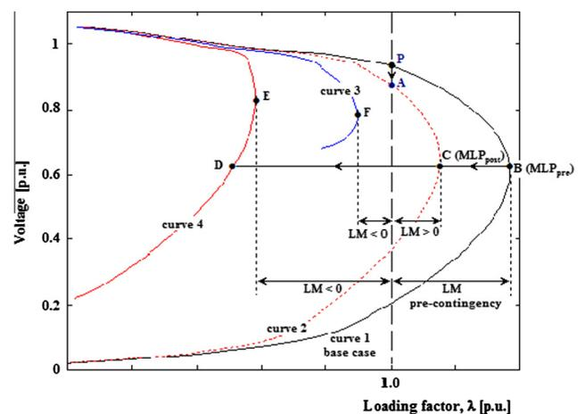
Fig. 1.  $P$ - $V$  curves for the base-case (pre-contingency) and for the outage of transmission lines.
