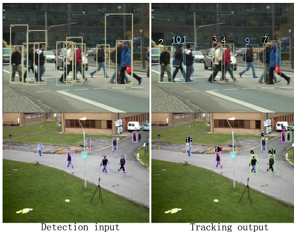
Fig. 1. Examples of detection input (left) and tracking output yielded by our approach (right). The input observations have a lot of false positives and false negatives. Besides, the box size and positive often do not fit the object. Our approach can remove the false positives and repair the missing detections.
