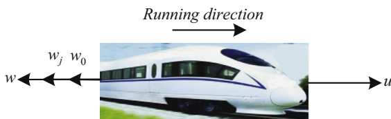
Fig. 1. Force analysis of the EMU's running process.
