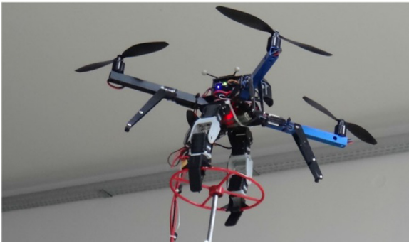
Fig. 1. Valve turning operation by a UAM [26].
