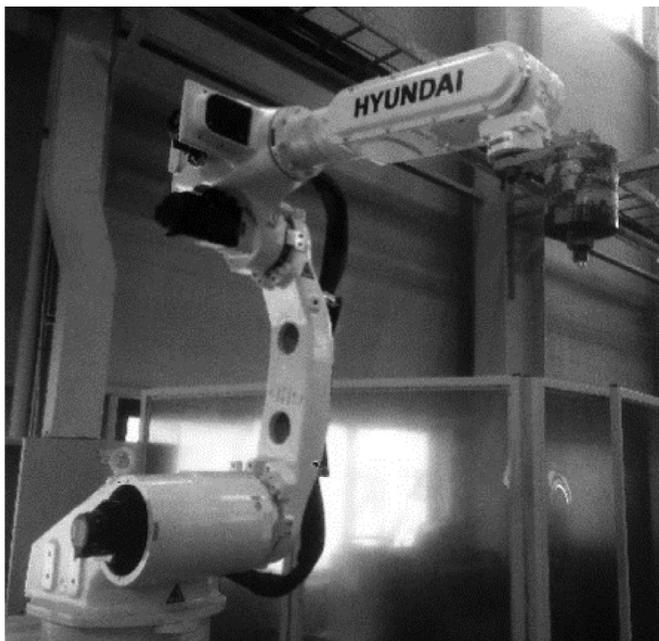
Fig. 1. HA006B (Hyundai industrial robot, DOF: 6, maximum payload: 6 kg, gearboxes of main axes: Nabtesco™ RV series, <http://www.hyundai-robotics.com/robot/robot01.asp>).
