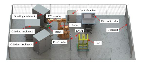
Fig. 1. The schematic diagram of the RBGS.
