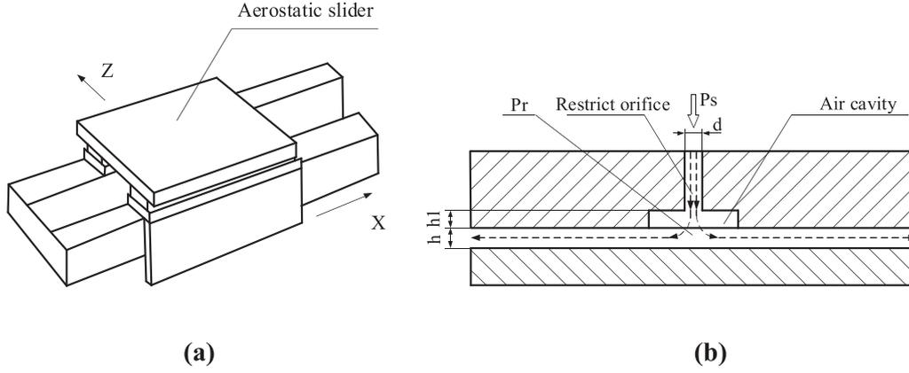
Fig. 1. (a) Configuration of the guideway; (b) air cavity of the aerostatic slider.
