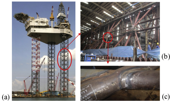
Fig. 1. The large and heavy workpiece in consideration: (a) The jackup oil rig consists of numerous legs; (b) The leg structure during fabrication; (c) The welded TKY joint. (Photograph courtesy of SembCorp Marine Limited, Singapore).
