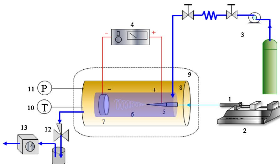
**Fig. 1.** Schematic diagram of the electrospinning system. (1. Polymer solution; 2. Syringe pump; 3. CO<sub>2</sub> cylinder & pre-heater; 4. High voltage power source; 5. Nozzle; 6. Polymer jet/fiber; 7. Collector; 8. PEEK autoclave; 9. Heater; 10. Temperature monitor; 11. Pressure gauge; 12. Back Pressure Regulator (BPR); 13. Flow-meter).
