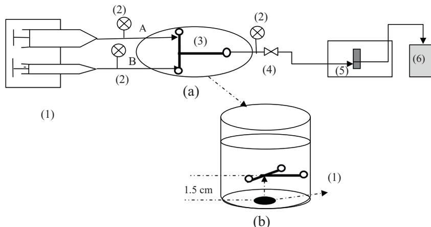
**Fig. 1.** A schematic diagram of the experimental setup: (a) – (1) syringe pump, (2) pressure sensor, (3) microchannel, (4) valve, (5) spectrophotometer, (6) product container and (b) container ultrasonic – (1) piezoelectric transducer 1.7 MHz.
