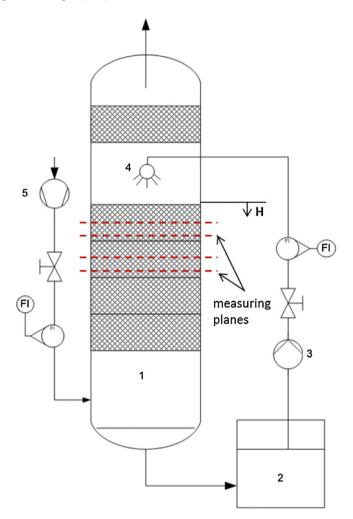
**Fig. 1.** Schematic flow sheet of the column setup. (1) Acrylic glass column; (2) liquid tank; (3) liquid pump; (4) liquid phase distributor; (5) air compressor. Dotted lines indicate the measuring planes.
