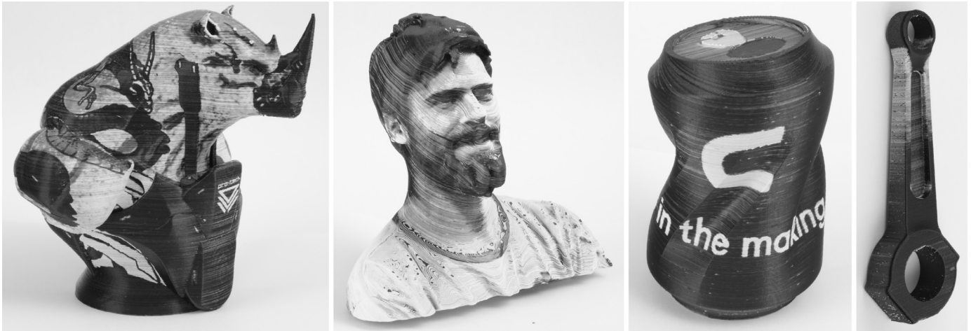
Fig. 1. 3D prints obtained by applying hatching on a 14 cm 3D portrait, a 15 cm artistic figurine, a full size soda can with textual information, and the result of a stress analysis performed on a 16 cm connecting rod of a piston engine.
