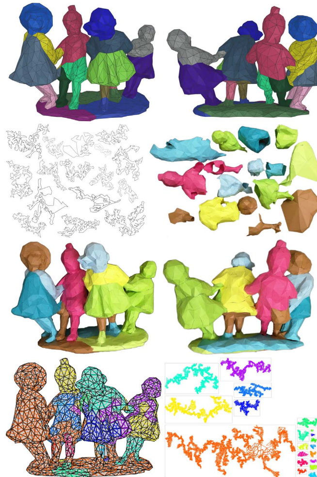
Fig. 2. Top row: the “Dancing Children” statue (3000 triangles) is segmented into 16 parts by the proposed method. Most of these parts corresponds to the heads, torso, legs of the model. The unfolded nets are shown in the middle. Second row: nets and the folded parts. Third row: a crafted paper model, which is about 30 cm wide, 11 cm deep and 22 cm tall. Bottom row: an optimization method proposed by Takahashi et al. [12] segments the same model into 21 nets that do not provide semantic information.
