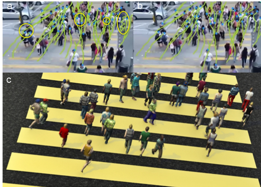
Fig. 1. (a) Pedestrian tracking using a simple particle filter and motion model. Yellow circles indicate some of the problems with prior tracking results, e.g. missing or incorrect tracks (b) Tracking using our algorithms with improved accuracy and smooth trajectories. (c) Rendering of the pedestrian trajectories from our data-driven crowd simulation system.
