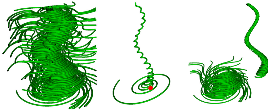
Fig. 1. Given an input pool of streamlines (left), we first segment each streamline using our previously learned classifier for segmentation points (middle, the red point is the segmentation point found by our algorithm). Partial streamline features specified by users will be clustered based on their similarities (right). (For interpretation of the references to color in this figure caption, the reader is referred to the web version of this paper.)
