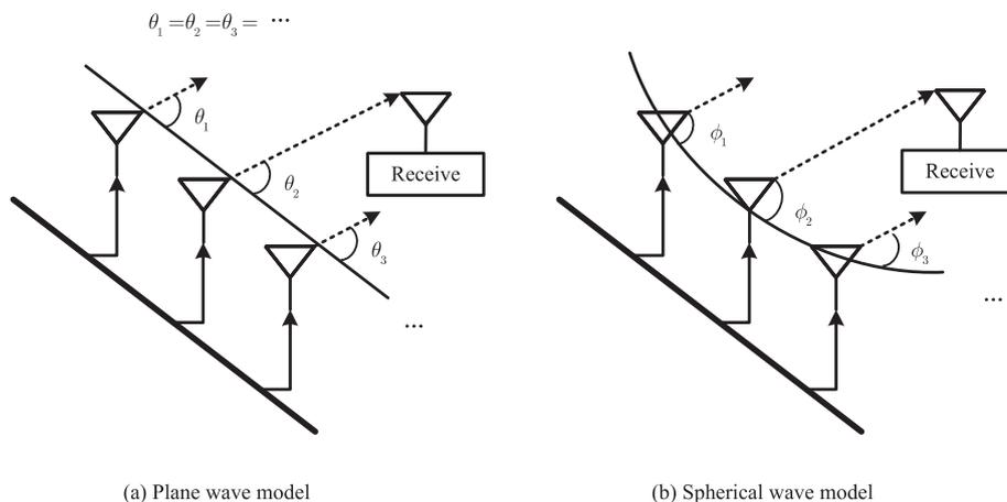
Fig. 1. Description of (a) the plane wave model and (b) the spherical wave model.
