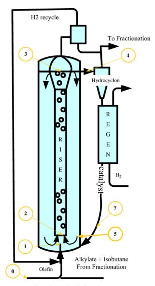
Fig. 1. Spouted bed-hydrocyclon system.
