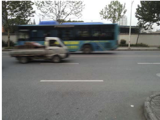
Fig. 1. The spatially-varying motion blur image: the moving objects are blurred and the background images are sharp.
