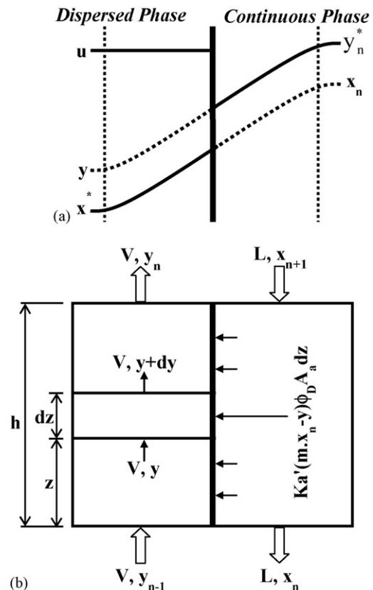
Fig. 1. Concentrations of excess dispersed phase reactant ( $u$ ) and solute ( $x$  and  $y$ ) across the interface at plate ( $n$ ).
