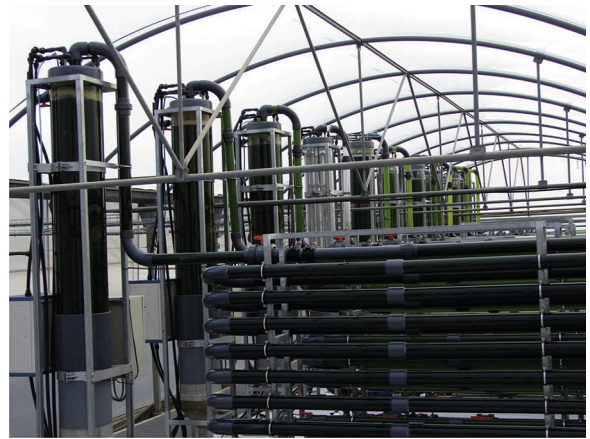
Fig. 1. A real view of 10 tubular photobioreactors at “Las Palmerillas” experimental station, Almería (Spain), showing the bubble column and the solar loop.
