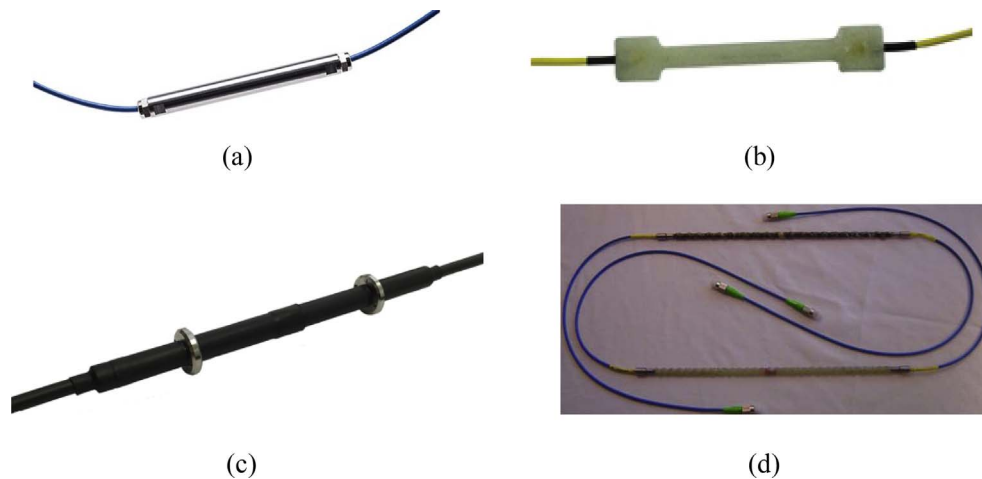
Fig. 1. The optical fiber based sensors used in practical engineering: (a) Steel packaged FBG sensor developed by HBM; (b) GFRP packaged FBG sensor developed by SCAIME; (c) Stainless steel packaged FBG sensor developed by MOI (d) CFRP/GFRP packaged FBG sensor developed by TELL.
