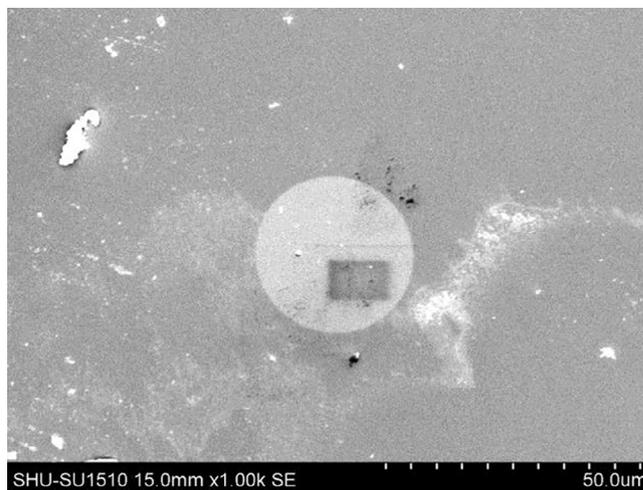
Fig. 2. The cross-section of the Si core fiber annealed at 1200  $^{\circ}\text{C}$ .
