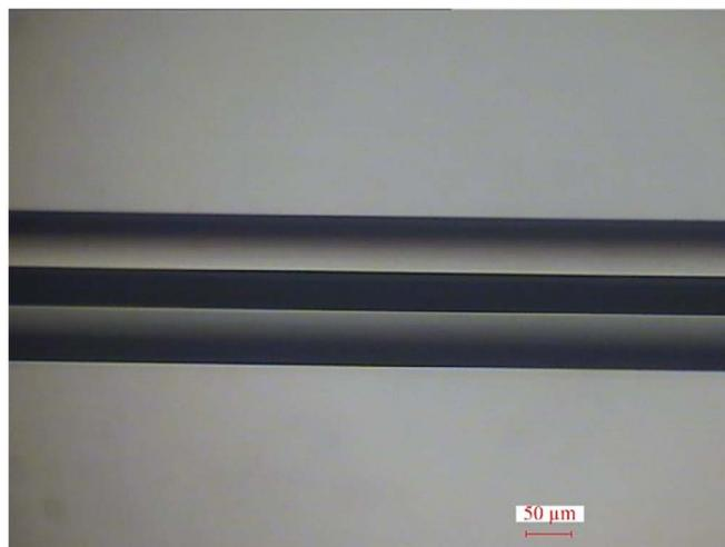
Fig. 1. The microscope photograph of the as-drawn Si core fiber.
