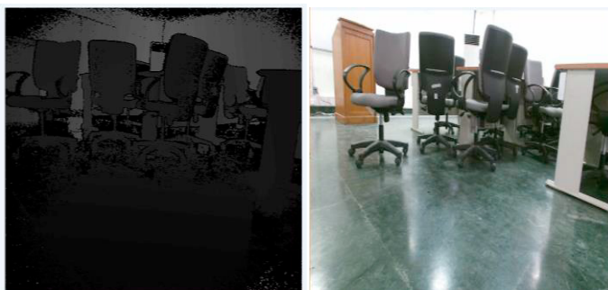
Fig. 2. Depth image and RGB image captured by Kinect v2 camera
