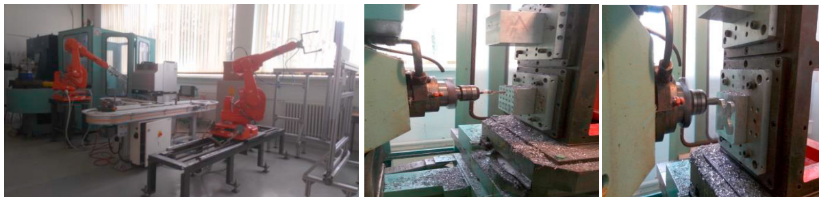
Fig. 1. Example of (a) Flexible manufacturing cell from Faculty of Managerial and Technological Engineering, University of Oradea, (b) Drilling processing, (c) Contour processing
