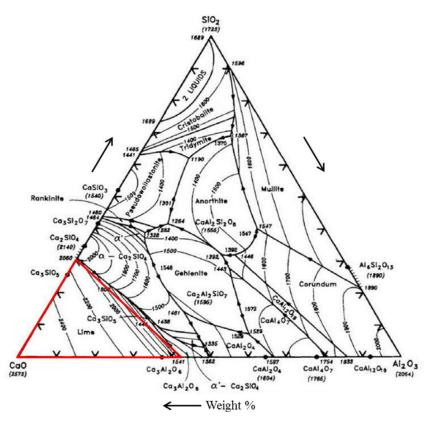
Fig. 1. A CaO-SiO<sub>2</sub>-Al<sub>2</sub>O<sub>3</sub> phase diagram (in °C) from literatures [20-22].
