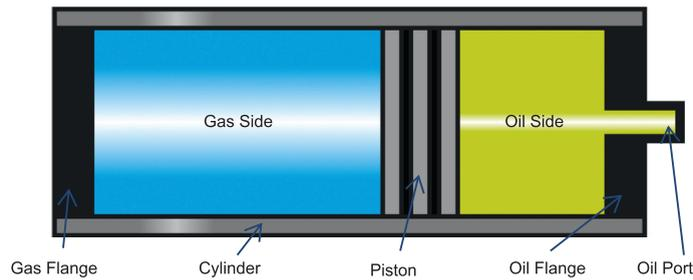
Fig. 1. Basic layout of a piston type hydraulic accumulator.
