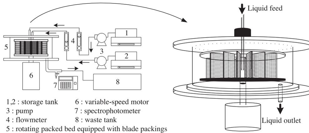
Fig. 2. Experimental setup for measuring micromixing efficiency.
